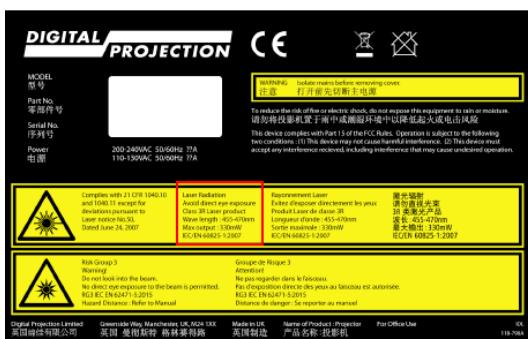
According to IEC 62471-5, the risk assessment of the projector light shall be carried out with the projector set to maximum brightness or maximum radiance emission. Projectors with non interchangeable lenses should be set so that the lens allows the maximum amount of brightness out of the lens. Projectors with interchangeable lenses should be tested at a throw ratio equal to 2.0:1. If 2.0:1 is not available, then the next higher ratio should be used.
