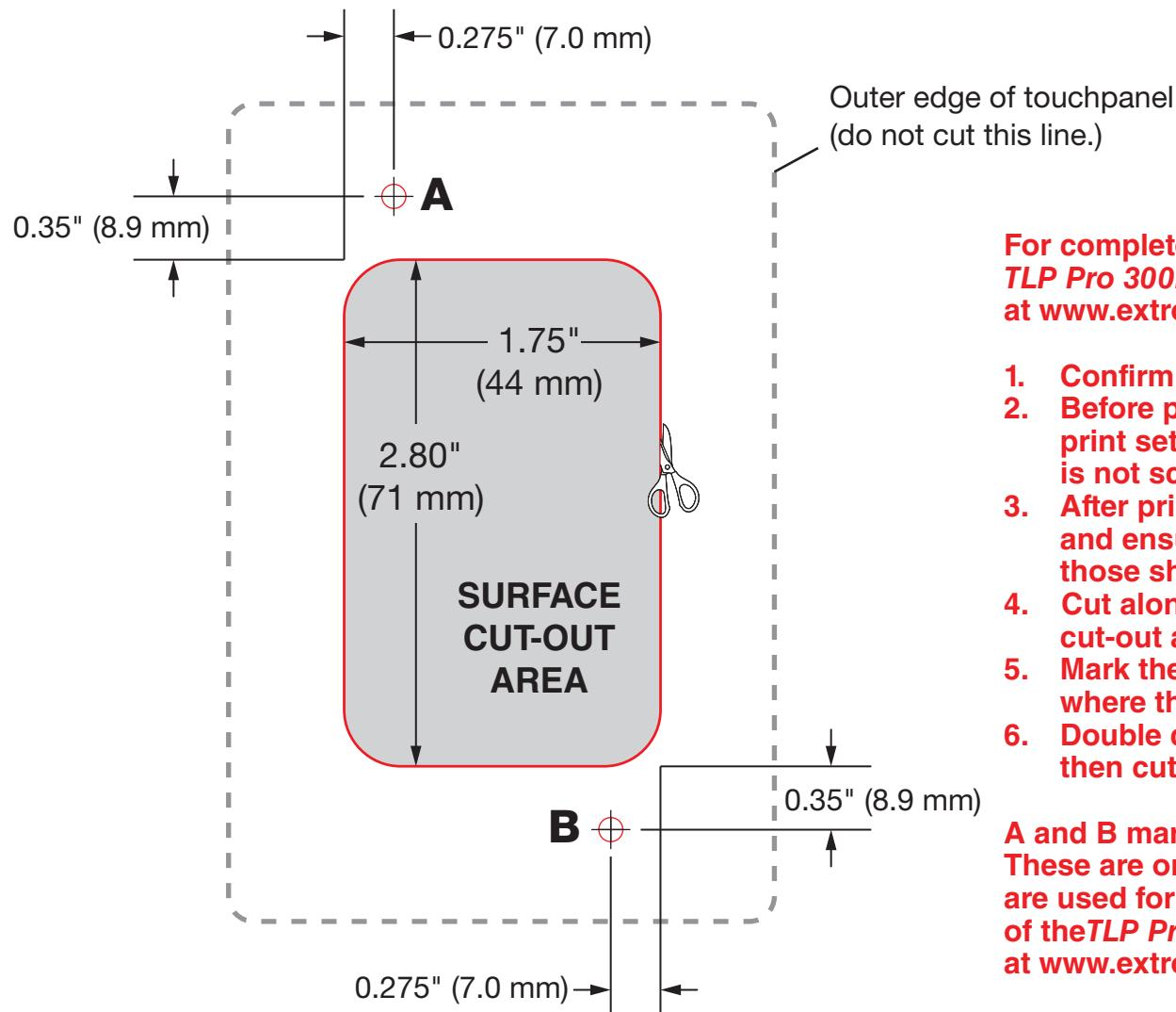
For complete installation instructions, see the *TLP Pro 300M Series Setup Guide* (available at [www.extron.com](http://www.extron.com)).
