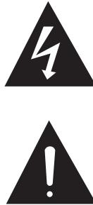
The lightning flash with arrowhead symbol, within an equilateral triangle, is intended to alert the use to the presence of uninsulated "Dangerous Voltage" within the product's enclosure that may be of sufficient magnitude to constitute a risk of electric shock to humans.
