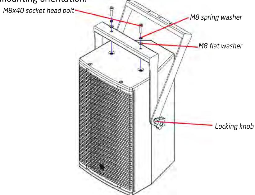
Loosen the locking knobs so that the outer yoke can be rotated relative to the inner yoke, which allows access to the mounting points. Line the yoke up, and using a 6mm Allen key, secure the yoke to the EMS-101X using M8x40 socket head machine screws, with flat and spring washers. Ensure the inner yoke is secure. The tilt angle can then be set with the locking knob.
