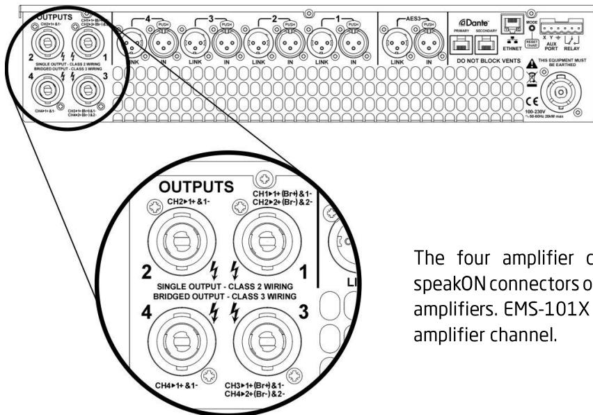
The four amplifier channels appear on four speakON connectors on the rear of the DQ Series amplifiers. EMS-101X loudspeakers require one amplifier channel.
