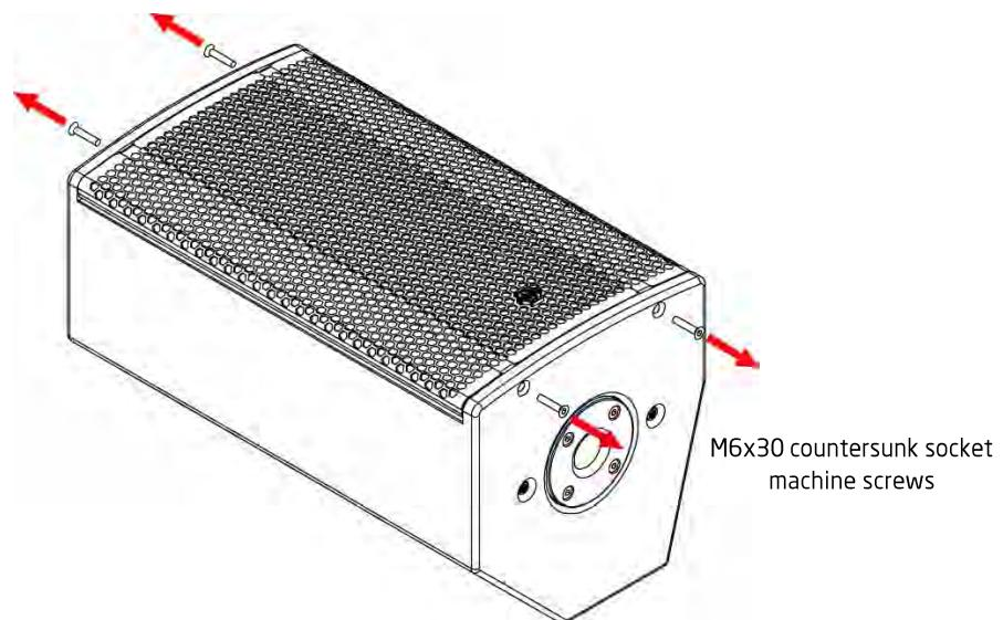
2. To replace the grille, position the grille on the front of the EMS-101X and ensure the threaded fittings on the grille are lined up with the mounting holes - gentle pressure may be required. Replace all of the M6x30 countersunk socket screws and ensure they are all are started in their threads before beginning to tighten. Ensure they are all tightened evenly so that the grille sits straight and does not rattle. Be careful not to over-tighten as this will distort the grille.
