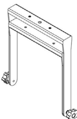
The FC-101Xv is a simple and effective means of mounting the EMS-101X in both temporary and permanent applications.
