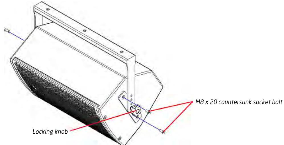
Ensure that all four bolts are properly tightened. Tighten the knobs on both sides to lock the desired angle for the EMS-101X.
