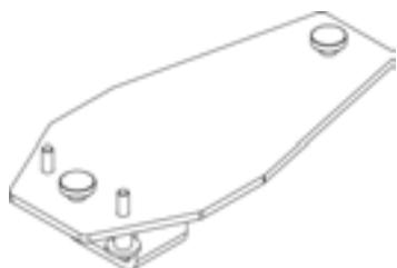
The CM-159 is designed to provide a means of mounting another loudspeaker directly below a flown MSE-159, in a safe and neat manner.
