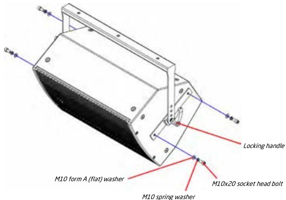
Ensure that the washers are in the correct order - form A (flat) in contact with the frame, and then the spring washer between the flat washer and the locking handle. Tighten the handles on both sides to lock the desired angle for the EMS-129.
