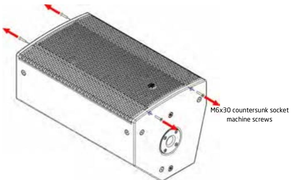
2. To replace the grille, position the grille on the front of the EMS-129 and ensure the threaded fittings on the grille are lined up with the mounting holes - gentle pressure may be required. Replace all of the M6x30 countersunk socket screws and ensure they are all are started in their threads before beginning to tighten. Ensure they are all tightened evenly so that the grille sits straight and does not rattle. Be careful not to over-tighten as this will distort the grille.
