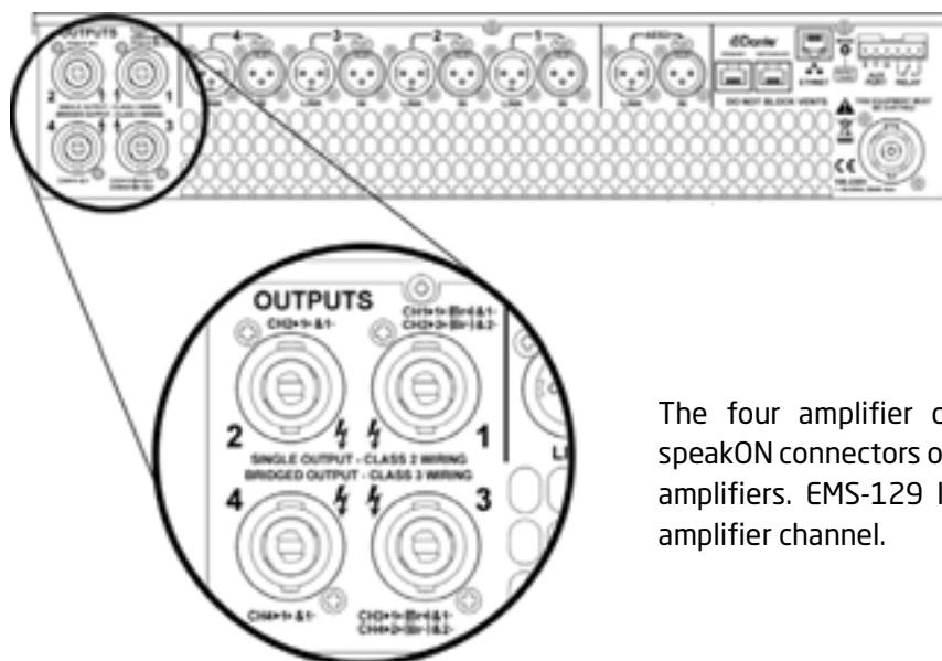
The four amplifier channels appear on four speakON connectors on the rear of the DQ Series amplifiers. EMS-129 loudspeakers require one amplifier channel.
