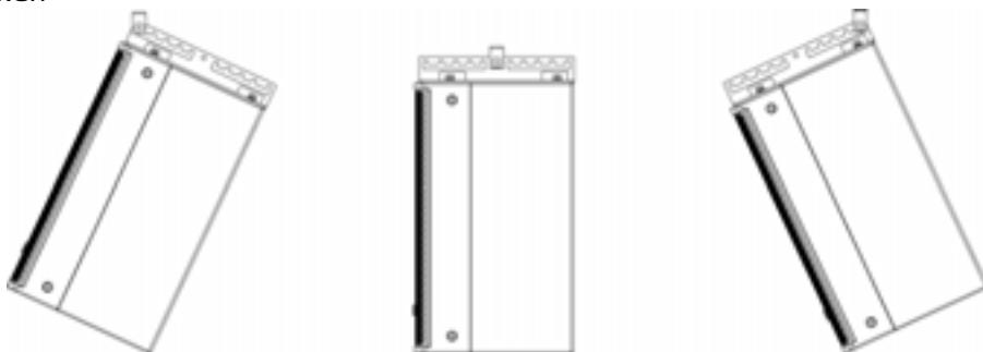
The central hole in the spine is for 0-degree flying. The track to the front is for up-tilt, and the track to the rear is for down-tilt - both in 5-degree increments.
