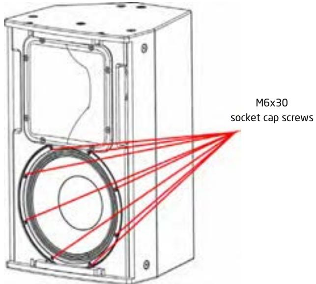
3. Lift the drive unit clear of the mounting hole and disconnect the cables - note the polarity for reconnection (brown to LF positive, blue to LF negative).
