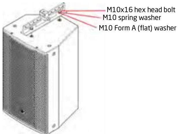
Secure the VFA-129 to the top of the EMS-129 using M10x16 hex head bolts, with spring and Form A (flat) washers. Ensure that both bolts are tight before attempting to lift the loudspeaker.
