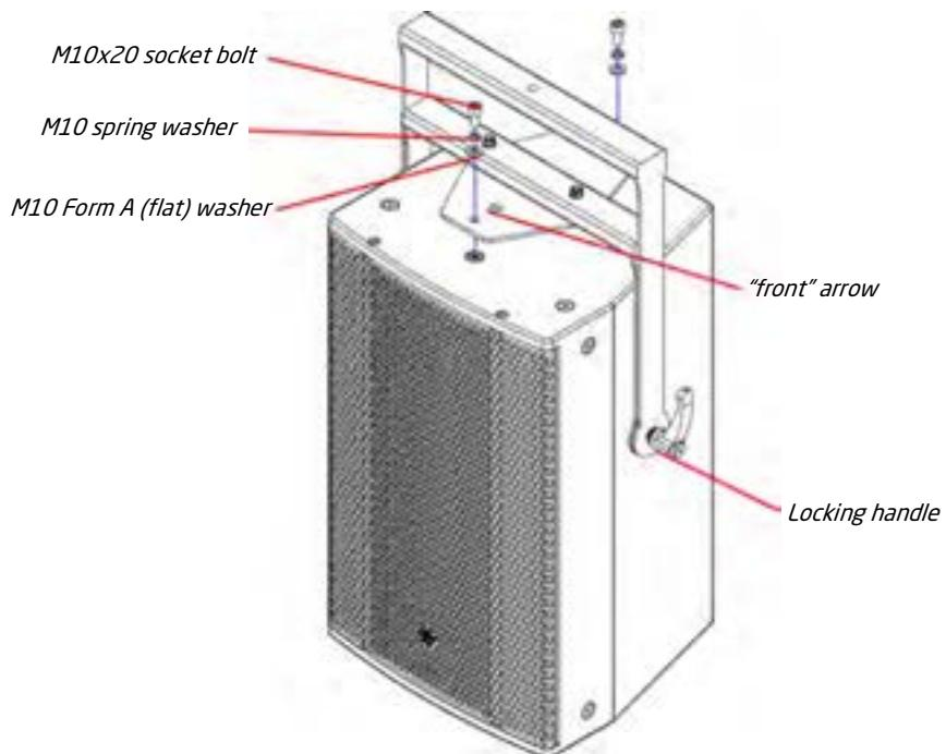
Using a 6mm Allen key, secure the yoke to the EMS-129 by bolting the mounting plate to the cabinet using M10x20 socket head bolts, with both spring washers and Form A (flat) washers. Ensure that the washers are in the correct order - form A (flat) in contact with the frame, and then the spring washer between the flat washer and the locking handle. Ensure the mounting plate is secure.
