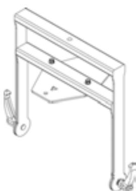
The FC-129v is a simple and effective means of mounting the EMS-129 in both temporary and permanent applications.
