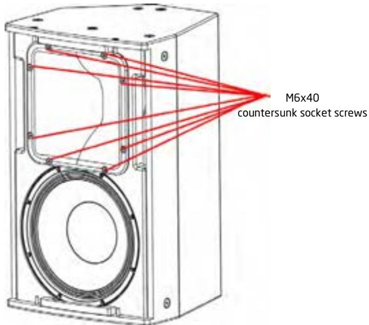
3. Lift the drive unit clear of the baffle and disconnect the cables - note the polarity for reconnection (white to positive, yellow to negative).
