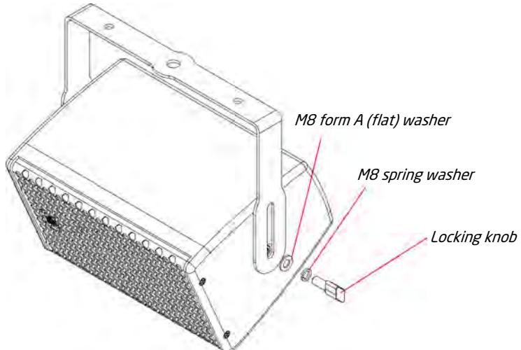
Ensure that the washers are in the correct order - form A (flat) in contact with the frame, and then the spring washer between the flat washer and the locking knob. Tighten the knobs on both sides to lock the desired angle for the EMS-51X.
