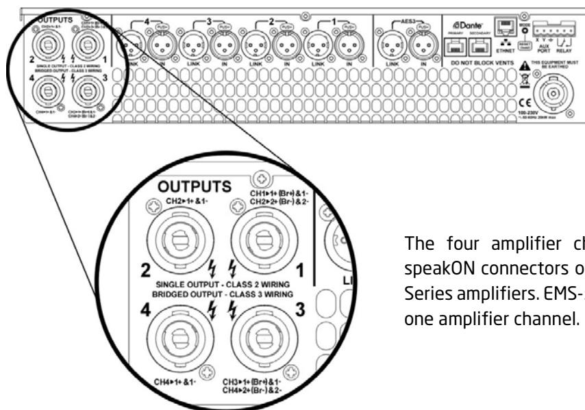
The four amplifier channels appear on four speakON connectors on the rear of the DQ & Di Series amplifiers. EMS-51X loudspeakers require one amplifier channel.
