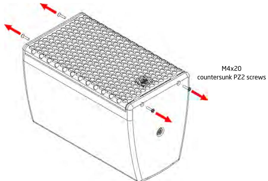
2. To replace the grille, position the grille on the front of the EMS-51X and ensure the threaded fittings on the grille are lined up with the mounting holes - gentle pressure may be required. Replace the four M4x20 countersunk screws and ensure they are both started in their threads before beginning to tighten. Ensure they are all tightened evenly so that the grille sits straight and flat and does not rattle. Be careful not to over-tighten as this will distort the grille.
